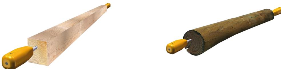
To evaluate the mechanical properties of structural wood, longitudinal measurements in direct mode are to be preferred.
